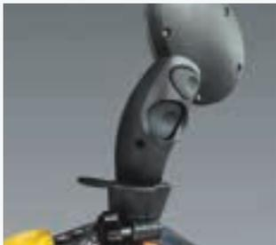
Shift button and ground speed unlock (behind)
