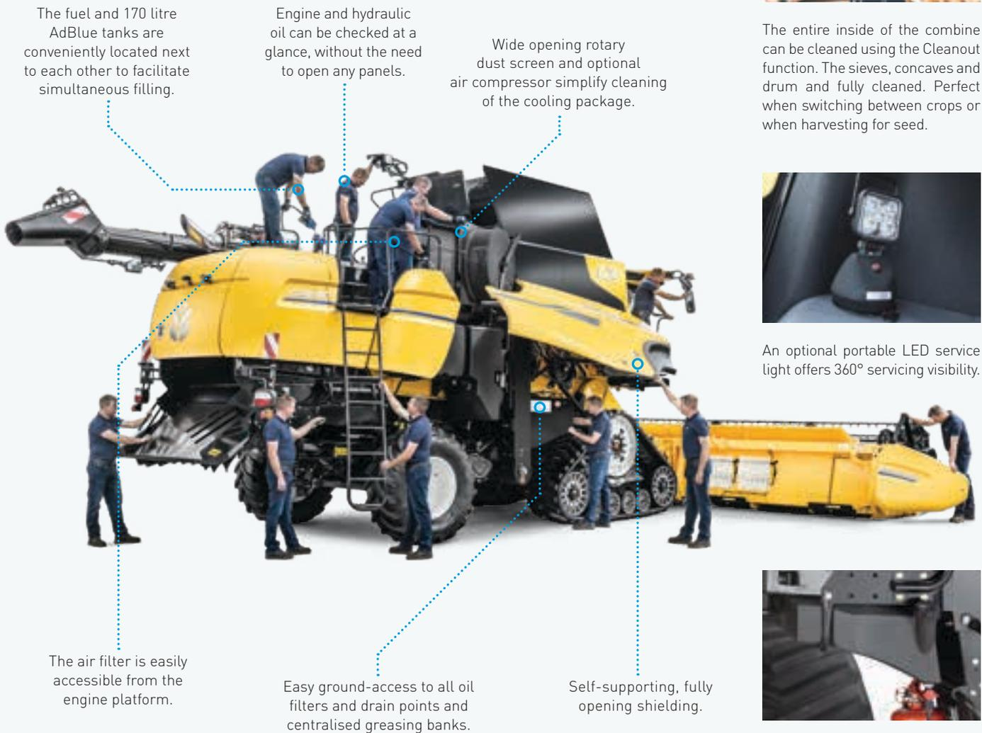
The fuel and 170 litre AdBlue tanks are conveniently located next to each other to facilitate simultaneous filling.
