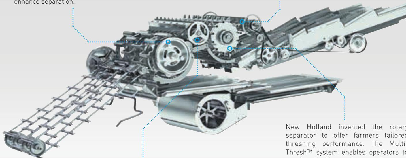
The beater's serrated teeth prevent mats forming in the crop to improve crop flow in all conditions, especially when harvesting marginal crops at high moisture levels.
