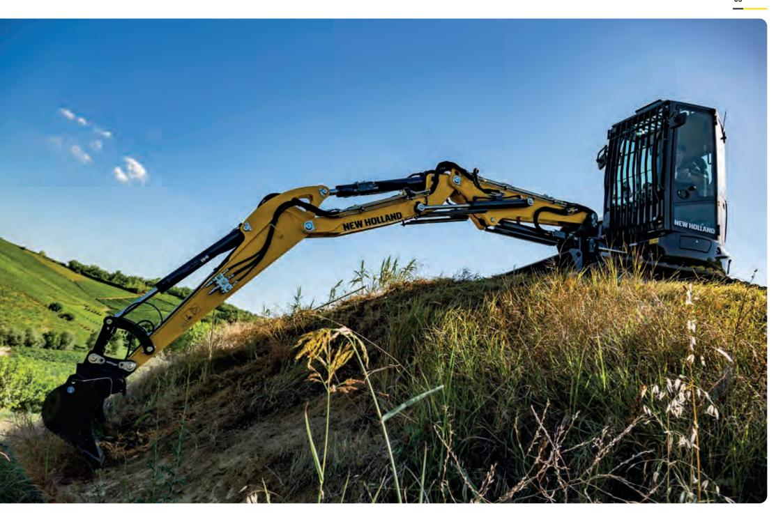
With only 790mm overall width, E12D and E14D can pass through a standard domestic door. Combined with a zero-tail swing for E12D and a short radius for E14D, these machines are designed to work anywhere.
