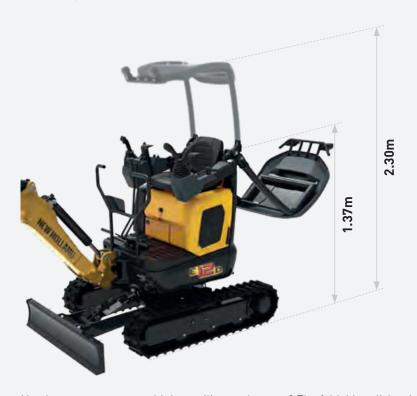
Need to access a room with low ceiling or doorway? The foldable roll-bar is easy to use, while also enabling compact machine storage without wasting building space.
