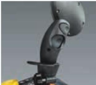
Shift button and ground speed unlock (behind).
