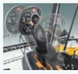
Force based movement enables the operator to change speed and direction.
